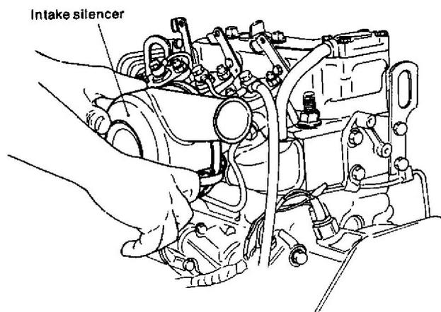
2-19. Remove the lifting hook at the rear of the engine together with the rear cylinder head cover
