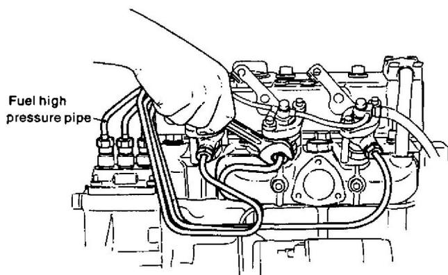
2-18. Remove the lifting hook at the front of the engine [3GM(D), 3HM]
