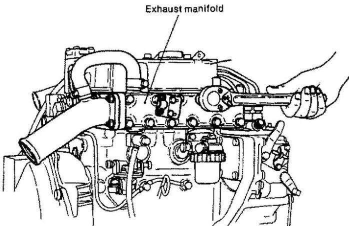
**2-8. Remove the cooling water pipe**
