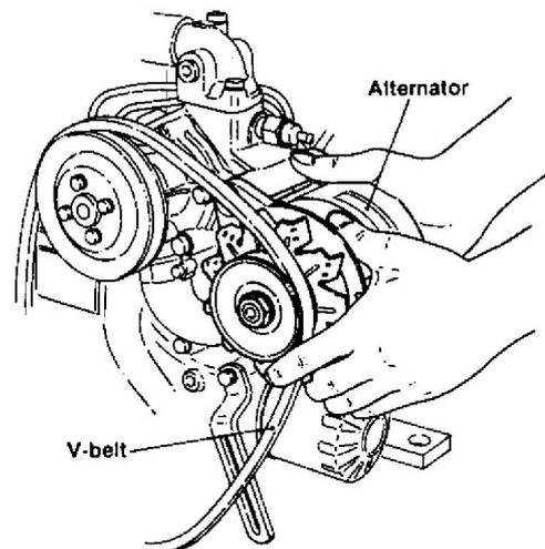
(2) Install the V-belt and tighten the adjusting bolt while adjusting the V-belt tension.
