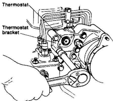
**2-14. Remove the cooling water by-pass connection**
