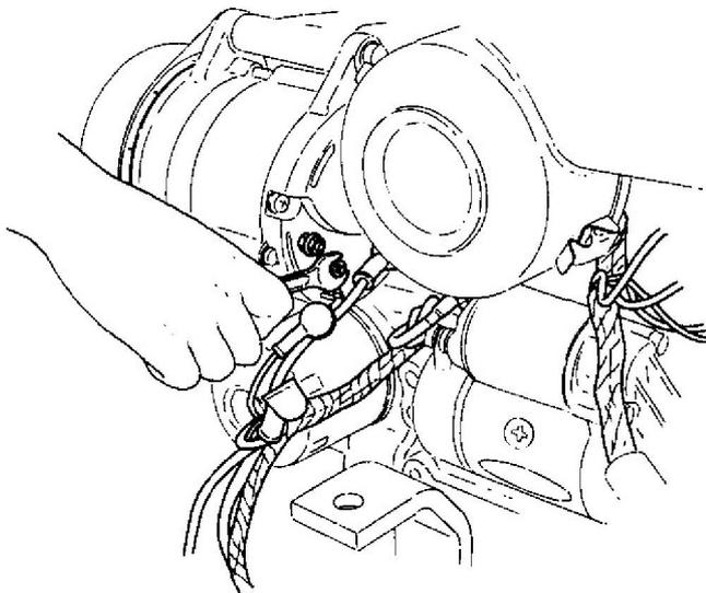
**2-12. Install the remote control cables**
