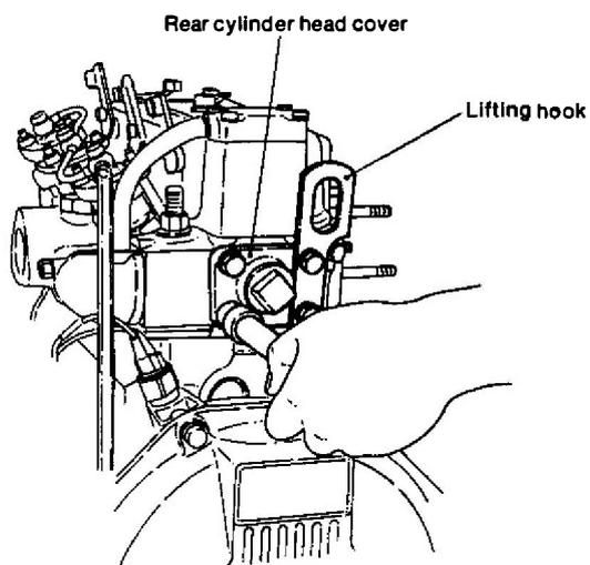
2-17. Remove the fuel high pressure pipe
