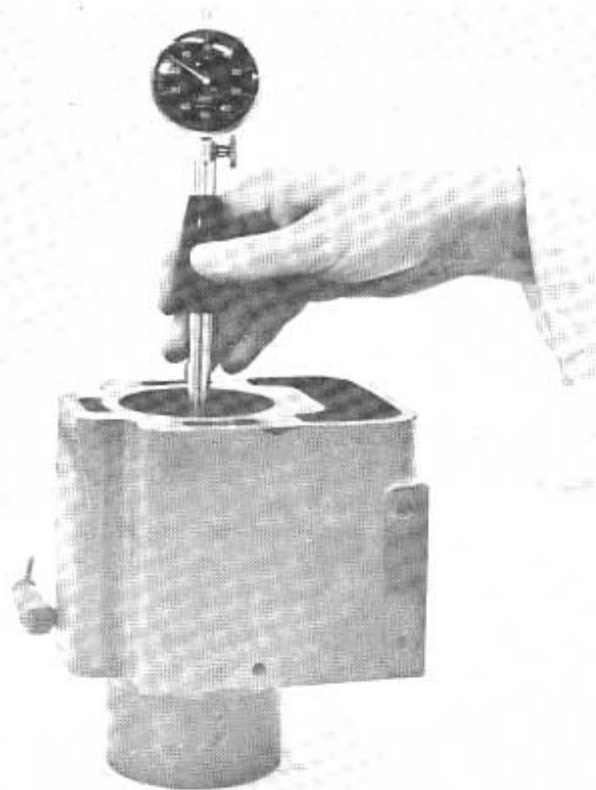
Fig. 17. Measuring cylinder bore wear
